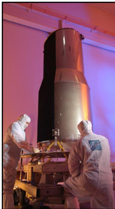
**Figure 3** – Spitzer CTA prior to protoflight environmental testing.
