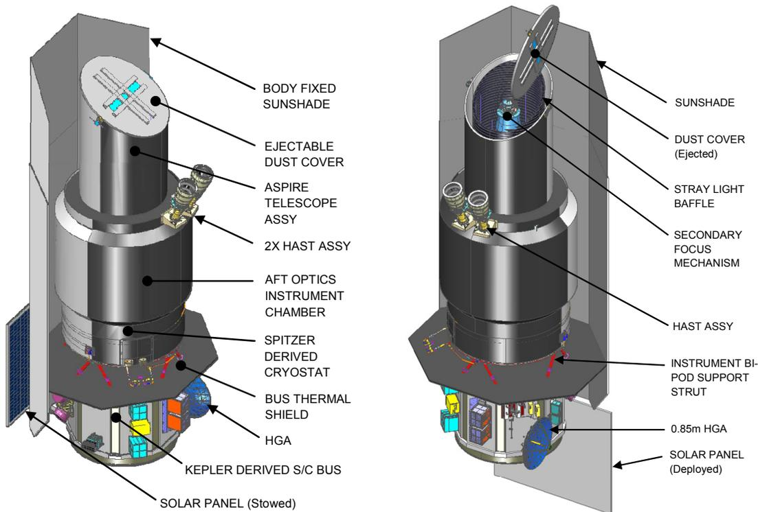
Figure 9 – The ASPIRE Observatory shown stowed (left) and deployed (right).
