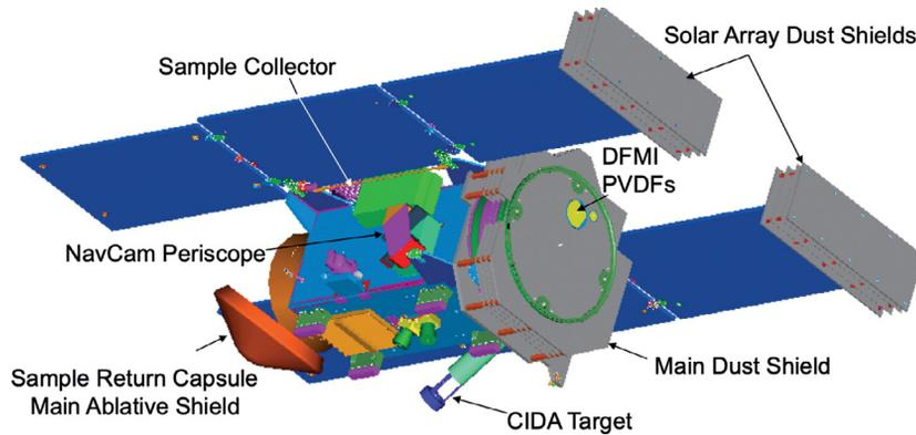
**Fig. 4.1** *Schematic of the Stardust spacecraft showing the positions of the onboard instruments.* The gray portions of the diagram represent the leading edge Whipple shields that protected the spacecraft from cometary dust impacts.
