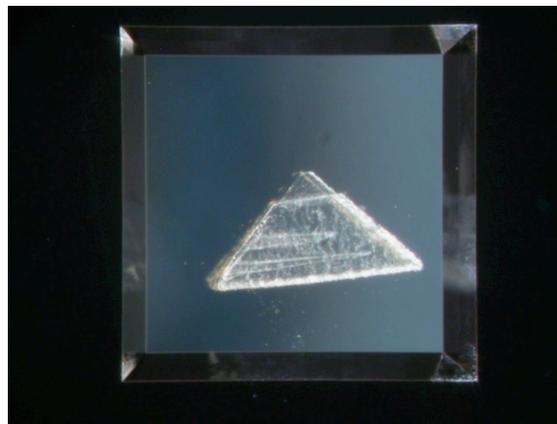
**FIGURE 2.** Picokeystone in a  $\text{Si}_3\text{N}_4$  sandwich. The window is 1.5mm square.
