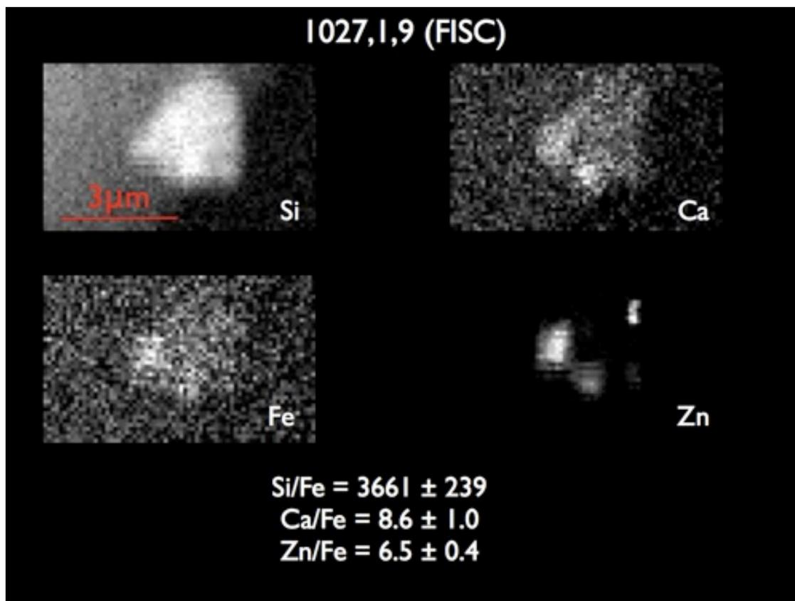
**FIGURE 5.** XRF maps of the first interstellar candidate, taken on ID22NI at the ESRF. The Ca/Fe, and Zn/Fe ratios are all significantly enhanced over CI values, indicating that it is unlikely to be of extraterrestrial origin.
