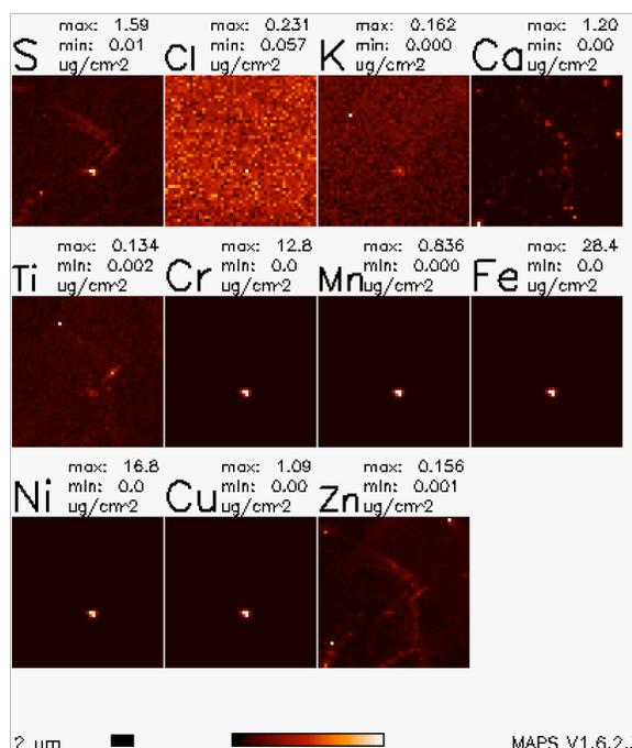
**FIGURE 6.** XRF maps of terminal particle in track I1004,1,2 taken on 2-ID-D at the APS. The Cr/Fe, Mn/Fe, Ni/Fe, and Cu/Fe ratios in this terminal particle are significantly enriched relative to cosmic abundances, and S/Fe, Ca/Fe, and Ti/Fe are all significantly below cosmic abundances.
