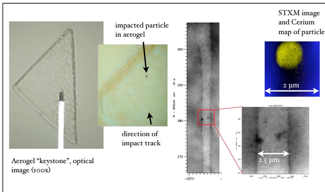
**FIGURE 8.** Absorption images (877 eV) of a portion of track I1017,2 in aerogel, taken on the STXM beamline 11.0.2 at the ALS.
